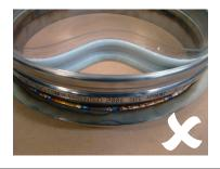
All care must be taken to ensure that the circumference of the head after fitting and welding remains the same size as supplied, to ensure fitting tolerance of the connector.
