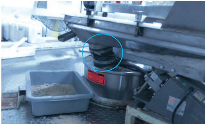
VIBRATORY SCREEN DISCHARGE TO AUGER FEEDER INLET - BEFORE
