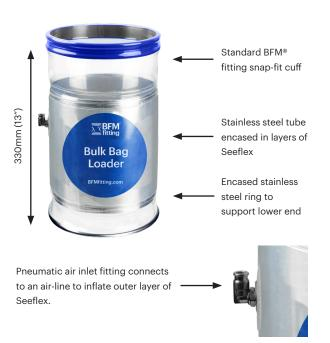
**NOTE:** If using in Atex Dust Zones, the up-line pipework and pneumatic air-line inlet fitting should be earthed.
