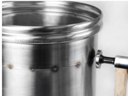
**05.** Peen the tacked joint to ensure correct fit.
