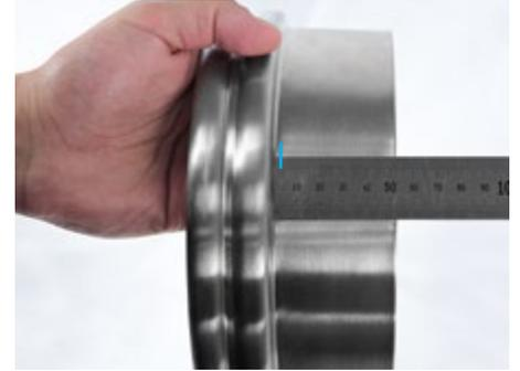
**03.** Avoid cutting the tail down if possible. If it is necessary to shorten it, we recommend leaving at least 15mm (½") on the tail.
