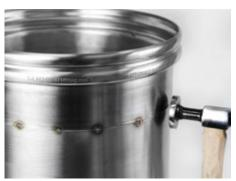
Peen the tacked joint to ensure correct fit.
